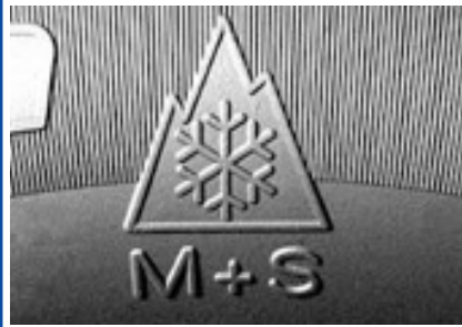
Snow tyres provide even better traction and are highly recommended (with the mountain/snowflake symbol pictured above)
